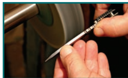
A 400-grit soft muslin wheel and a light touch is one way to keep those serrations sharp.
