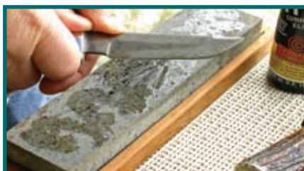
Above: A piece of non-slip mat will hold that stone in place, permitting both hands on the knife for better control.
