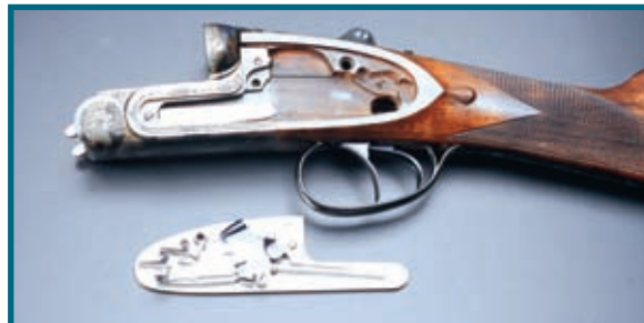
Detachable sidelocks must be perfectly fitted to both metal and wood. The seven pins that make these so distinctive are actually screws that hold the lock parts onto the side plate. The lock inletting is also just as beautiful.
